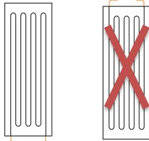
When the panel is installed in vertical position, always the inlet and outlet connection has been at the bottom (it is not allowed to install the reverse).
