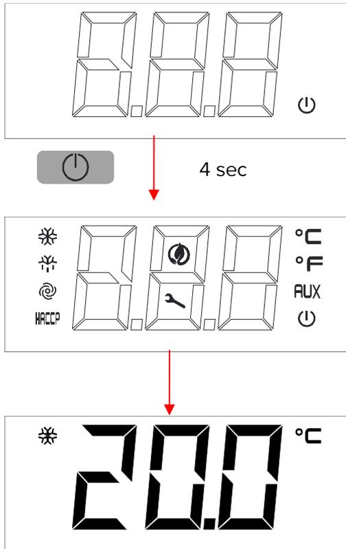
1. After filling the tank of water, connect the mains plug to the mains supply. The screen will show the
