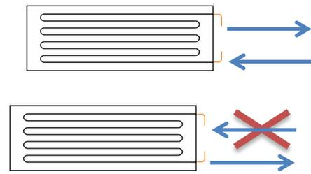
If the panel is installed at horizontal position, refrigerant inlet pipe should be connected into the bottom connection.
