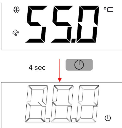
To switch off the system, hold the
